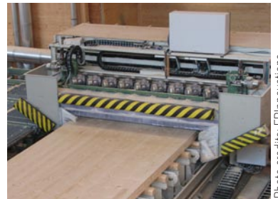
Manufacturing of cross laminated timber.
